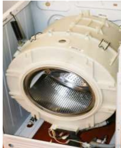
Outer Drum (Vibration)
